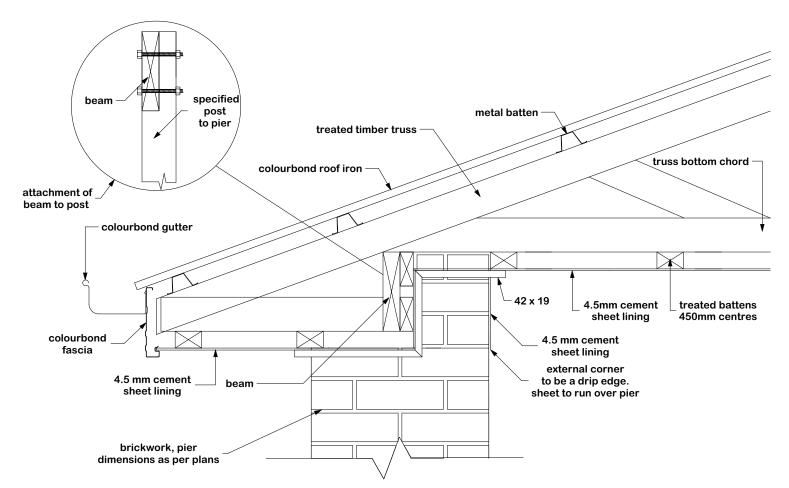
Brick Pier & Lined Eave Lower Than Ceiling Detail SCALE NTS
